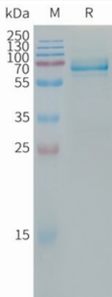
Figure 1. Human LILRB4 Protein, hFc Tag on SDS-PAGE under reducing condition.
