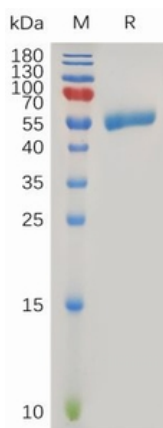
Figure 1. Human CLEC4C Protein, hFc Tag on SDS-PAGE under reducing condition.
